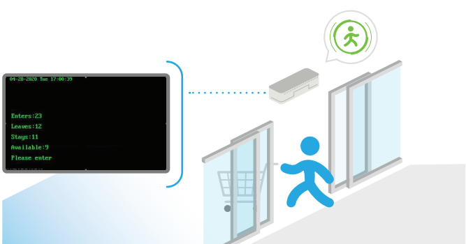
Single Door Camera Standalone Density Control Solution
